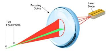
Diagram shows the problem of astigmatism, and how it can limit your optical system's performance in terms of focused beam shape and size. If precise beam placement or a small focused image is required by your system, astigmatism should be considered.
