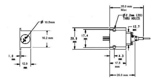
Fiber Pigtailed 532nm Laser Module
